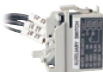
Auxiliary switch is for applications requiring remote "On" and "Off" indication. Each switch contains two contacts having a common connection. One is open and the other closed when the circuit breaker is open, and viceversa.
